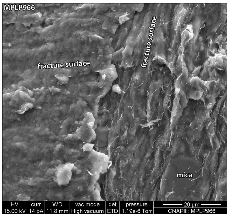
Plate 7.2.36: SE SEM image, sample MPLP966, C-coated rock chip. This site is where two fracture faces with different orientations of striae converge. Fibrous constituents are common.
