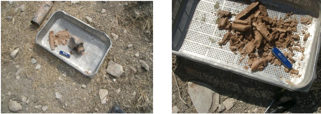
Figure 6.1.4: Bentonite/analogue bentonite core material from the boreholes at Parsata. Note Swiss Army Knife for scale is approximately 10 cm long.
