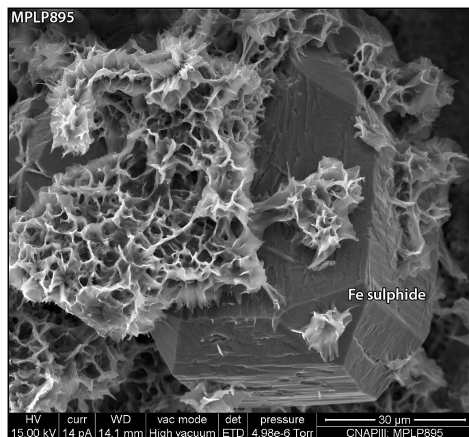
Plate 7.2.20: SE SEM image, sample MPLP895, C-coated rock chip. Webbed clays partially coating an iron sulphide crystal, both within a secondary pore. The surfaces of the sulphide crystal are finely stepped, notched and striated; whilst these are mostly growth textures there is some evidence of minor dissolution.
